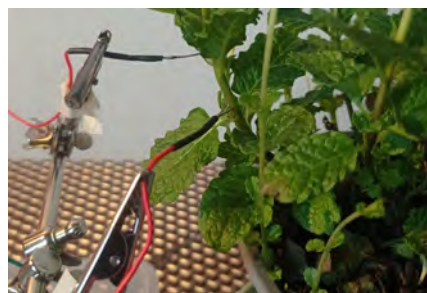
Fig. 5. Ag/AgCl electrode placed on Mentha spicata stem, visualisation with the Partiels software of the of the VP-like morphology acquired through Audacity. X axis represent the PCM amplitude and y axis the time in 00m:00s:000ms.
