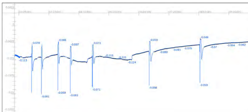
Fig. 4. Visualisation with the Partiels 10 software of the AP-like morphology acquired through Audacity. X axis represents the PCM amplitude and y axis the time in 00m:00s:000ms.
